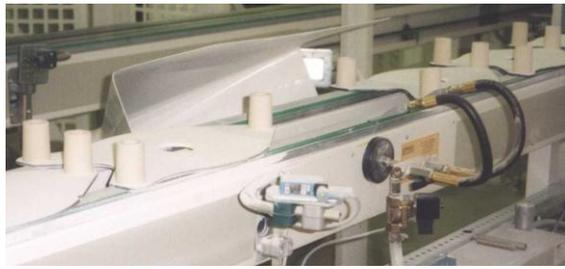
Fig. 2: Combined blowing/suction device for cleaning kiln furniture
