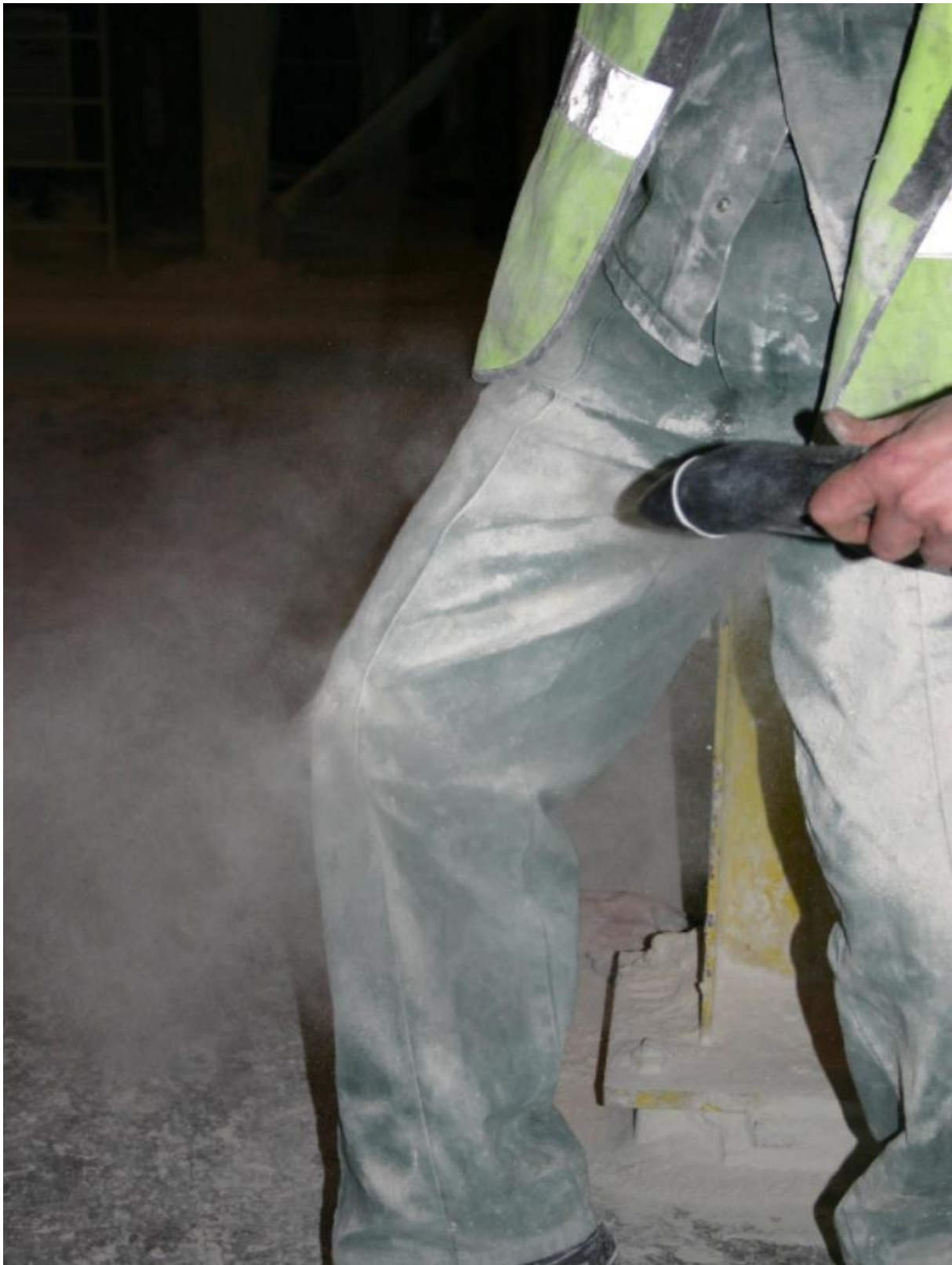
Fig. 1: Prohibited blowing off of dust using pressurised air
